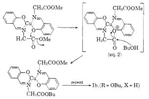
The mechanism involves an attack on the ester carbonyl linkage by the oxygen of the salicylaldehyde portion of the molecule to form an intermediate lactone type structure. This reaction would be expected to be reversible and reaction with the alcohol in excess, e.g., the alcohol used as solvent opens the intermediate to give the new ester.
