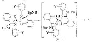
The aliphatic base attacks the electron deficient carbon at the polarized azomethine link. The driving force of the reaction may be attributed to the large excess of butylamine over the substituted aniline displaced, or to the greater basicity of the aliphatic amine.
